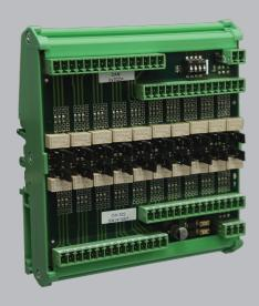
We have expanded our CW-300 series for test bench technology with the CW-322, a module designed to control up to 20 signal relays via CAN bus. This module not only supports targeted actuation of a single relay, but also synchronized control of several relay channels.
