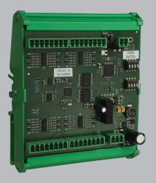
We have expanded our CW-300 series for test bench technology with the CW-327, a module designed to measure 16 analog voltages. It is possible to measure voltages from 0 to max. 60 VDC per channel with a 16 bit resolution. Device settings such as baud rate of the CAN bus, output transfer rate, voltage ranges and transmission modes can easily be configured via CAN messages. All 16 inputs are sampled synchronously and issued on the CAN bus.
