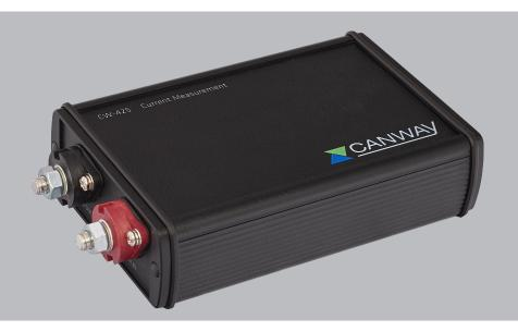
The CW-425 offers a simple possibility to obtain highly precise measurement of quiescent and operating current of devices (e.g. electronic control unit). It offers a total measurement range up to  $\pm 150$  A. Switch-over of measurement ranges is automatically performed within 1  $\mu$ s (quiescent current to load current) during ongoing operations.
