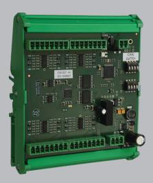
We have expanded our CW-300 series for test bench technology with the CW-327, a module designed to measure 16 analog voltages. It is possible to measure voltages from 0 to max. 60 VDC per channel with a 16 bit resolution. Device settings such as baud rate of the CAN bus, output transfer rate, voltage ranges and transmission modes can easily be configured via CAN messages. All 16 inputs are sampled synchronously and issued on the CAN bus.
