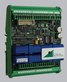
Utilizing the CW-328 it is possible to quickly and easily measure currents with very little effort. The addition to the CW-300 series from CANWAY is designed for test bench and other applications.
