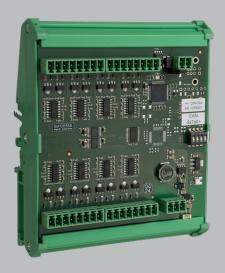
We have expanded our CW-300 series for test bench technology with the CW-324, a module with 16 sink mode outputs. It is possible to set each current sink between 0 and 20 mA with a high 12 bit resolution. Furthermore, the amperage can be redefined 100 000 times per second and all 16 channels synchronized.
