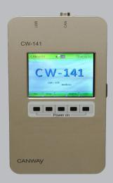
The CW-141 makes it possible to study and analyze CAN networks. Designed as a portable, hand-held device in a rugged aluminium housing, it is particularly suitable for mobile use.
