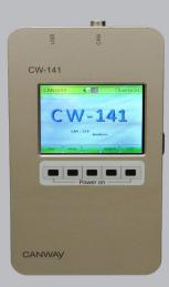
The CW-141 makes it possible to study and analyze CAN networks. Designed as a portable, hand-held device in a rugged aluminium housing, it is particularly suitable for mobile use.
