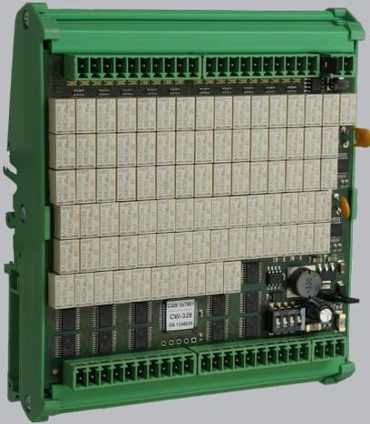
The Failure Injection Unit (FIU) serves to provoke physical failures, for example, to validate electronic control units. It is a further module belonging to the CW-300 series, that can be used to automate test environments on HiL test benches.
