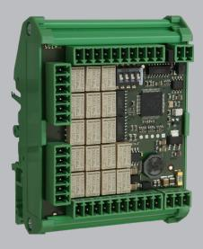
The bus and signal multiplexer module is a further product belonging to the CW-300 series for test bench technology and test bench automation. Utilizing the CW-325 it is possible to control the signal paths of bus systems such as CAN bus and FlexRay™ or any desired signal.
