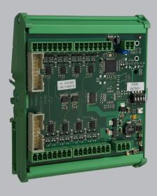
We have expanded our CW-300 series for test bench technology with the CW-323, a module designed to output 16 analog voltages. It is possible to freely select these voltages between 0-5 VDC with a high 12 bit resolution. The voltage outputs are controlled via the CAN bus. If required, it is possible to synchronize all 16 voltages.
