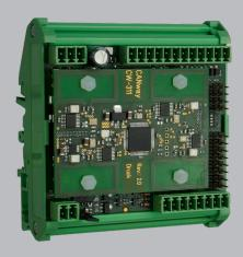
CW-311 wheel speed and wheel unit simulator allows to simulate tire pressure, tire temperature and wheel speed sensors, as commonly used in the automotive industry. Fields of application are HiL - test benches (hardware-in-the-loop) for ecu (electronic control units).
