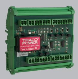
The CW-310 is designed for signal conditioning during simulation of active wheel speed sensors. To do so it emulates the physical layer of widespread wheel speed sensors available on the market.
