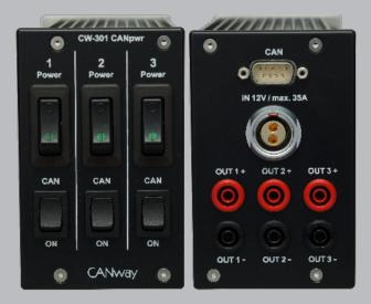
The module CW-301 makes it possible to switch power relays by means of CAN messages and manual switches. For instance, it can be used to switch on the power supply to mobile measuring equipment, by means of a specific CAN bus signal (e.g., KL15). Rather the CW-301 can used to charge measurement equipment batteries within defined vehicle states.
