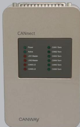
CANWAY's CANnect is a gateway for CAN and LIN busses. Following the original and popular CANnect 1's principles, the new model is a complete redesign based on state-of-the-art technology. Typical applications are for example stimulating different test objects in testbenches or integrating new ECUs and sensors in an existing car's network. Also, the CANnect provides extensive capabilities for generating signals and messages including bus protocols in order to simulate ECU prototypes.
