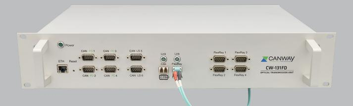
The CW-131FD Optical Transmission Unit provides bidirectional optical transmission of automotive network data over distances - up to 500 m. Overall, it is possible to connect 4 CAN FD/HS (flexible datarate/highspeed), 2 CAN LS (lowspeed) and 4 FlexRay™ (channel A and B) buses.
