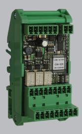
We have expanded our CW-300 series for test bench technology with the CW-329, a module designed to optionally control up to 3 signal relays via CAN bus or digital inputs. This module not only supports targeted actuation of a single relay, but also synchronized control of several relay channels.
